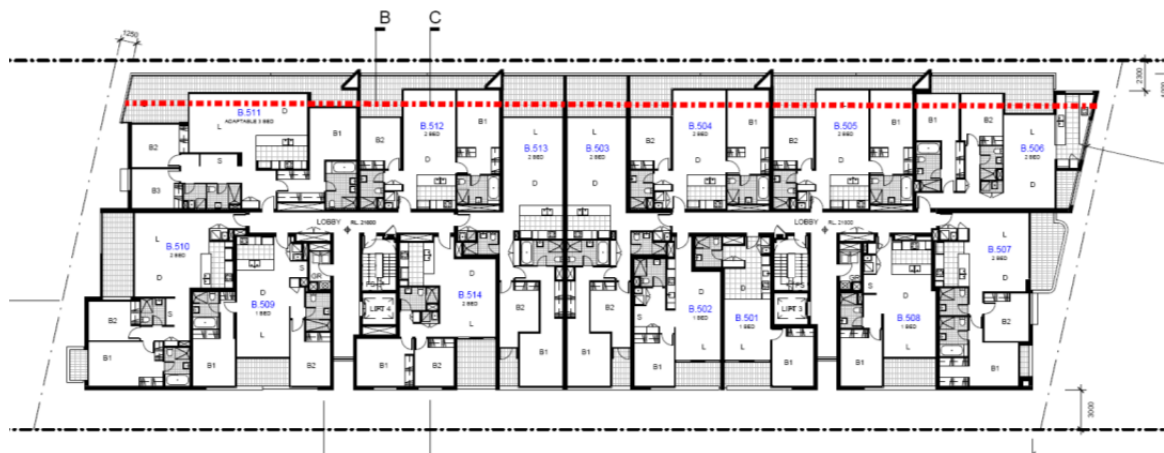
Figure 25 – Typical level, Building 2B. Original proposal showing extent of encroachments beyond the required setback, shown dashed. In the original proposal apartments and balconies projected beyond the allowed setback for almost 100% of the elevation.
