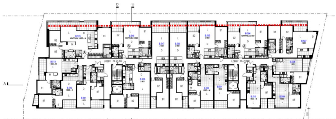
Figure 26 – Typical level, Building 2B. Amended proposal. The extent of projections has been reduced to 72%.
